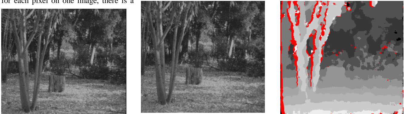
Figure 5: A stereo pair, and a resulting depth image. The red regions denote ambiguous depth without stereo matching not at all by the magnitude of the discrepancies.
